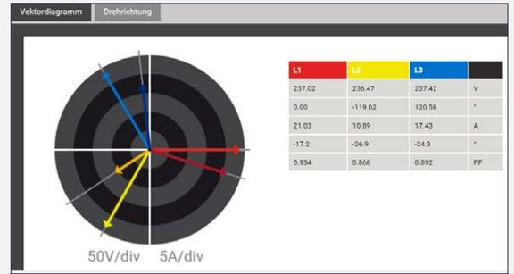
Phasor diagram to control connections
